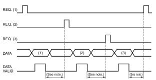
Note: Leave 20 ms min. between DATA VALID turning OFF and the REQUEST signal.
