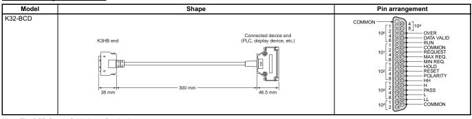
Note: The BCD Output Cable has a D-sub plug.
