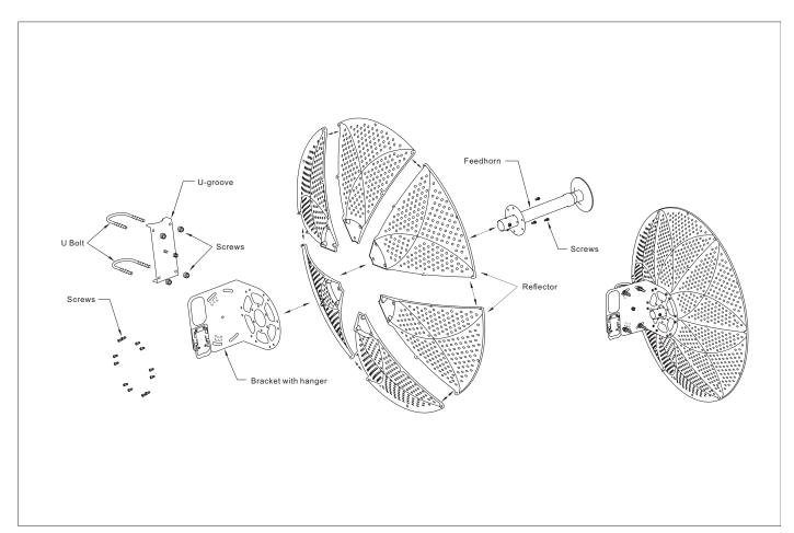
4950 MHz to 7125 MHz, 3-foot mesh collapsible Parabolic Antenna, 2x2 MIMO, 34 dBi, RPSMA, 2 Pack from L-com has same day shipment for domestic and International orders. Our portfolio includes coaxial cable assemblies, connectors, adapters and custom products as well as lightning and surge protectors, NEMA rated enclosures, and an RF product line which includes antennas, amplifiers, passive, and active components.
