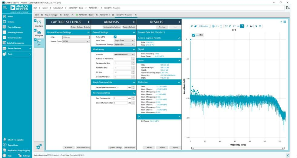
Figure 23. ADAQ7767-1 Board FFT Without Buffers
