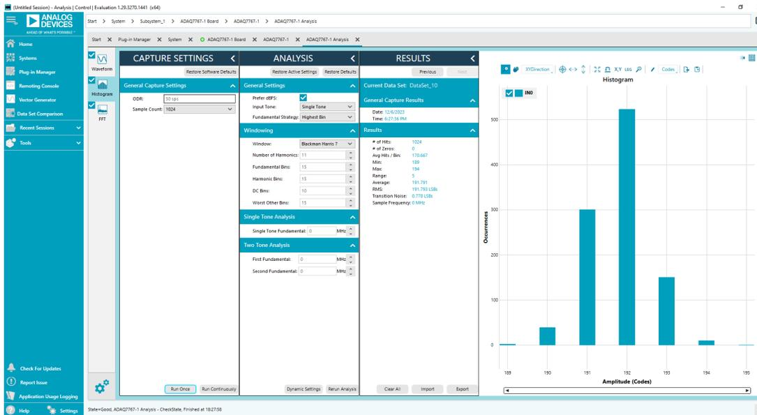
Figure 6. Histogram of Output Codes with IN2+ and IN2- Shorted to GND and Sinc3 = 50 SPS
