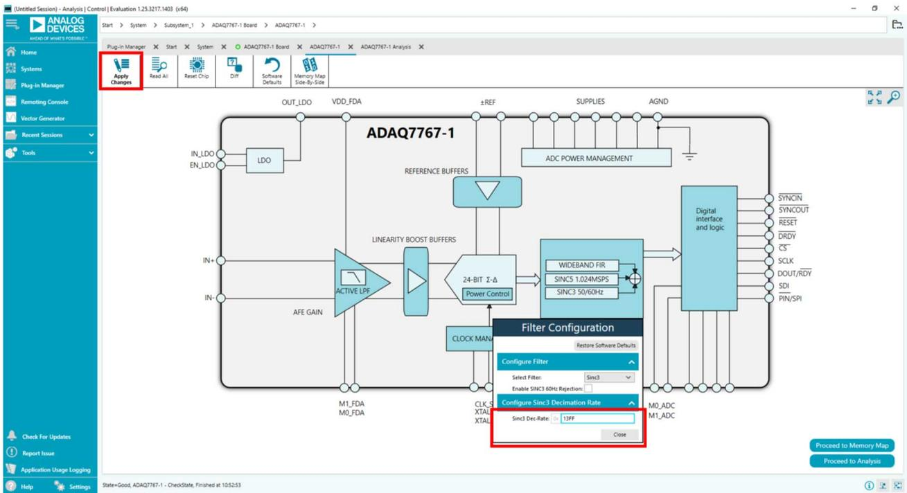
Figure 5. Set the Sinc3 Filter Decimation Ratio
