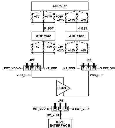
Figure 8. VDD\_BUF, VSS\_BUF, and HV\_VDD Jumper Settings
