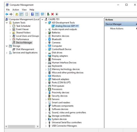
Figure 16. Checking That the Evaluation Board Is Connected to the PC Correctly
