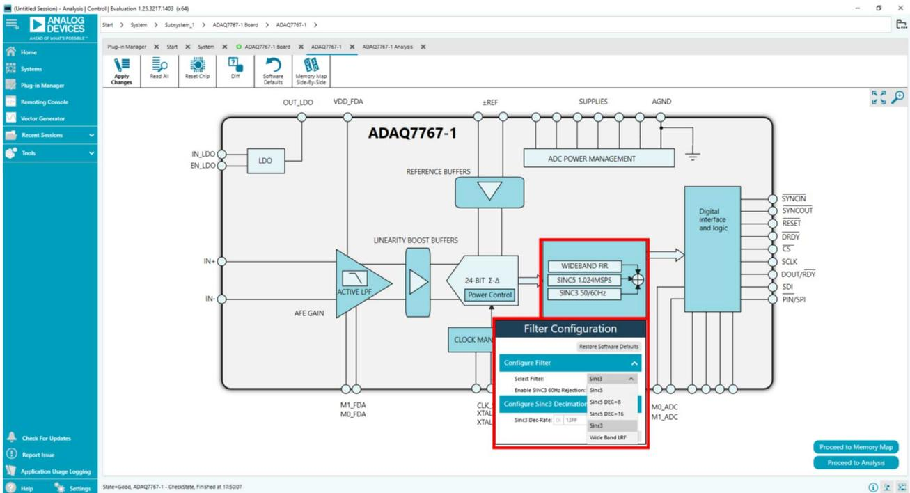
Figure 4. Set the Digital Filter Type
