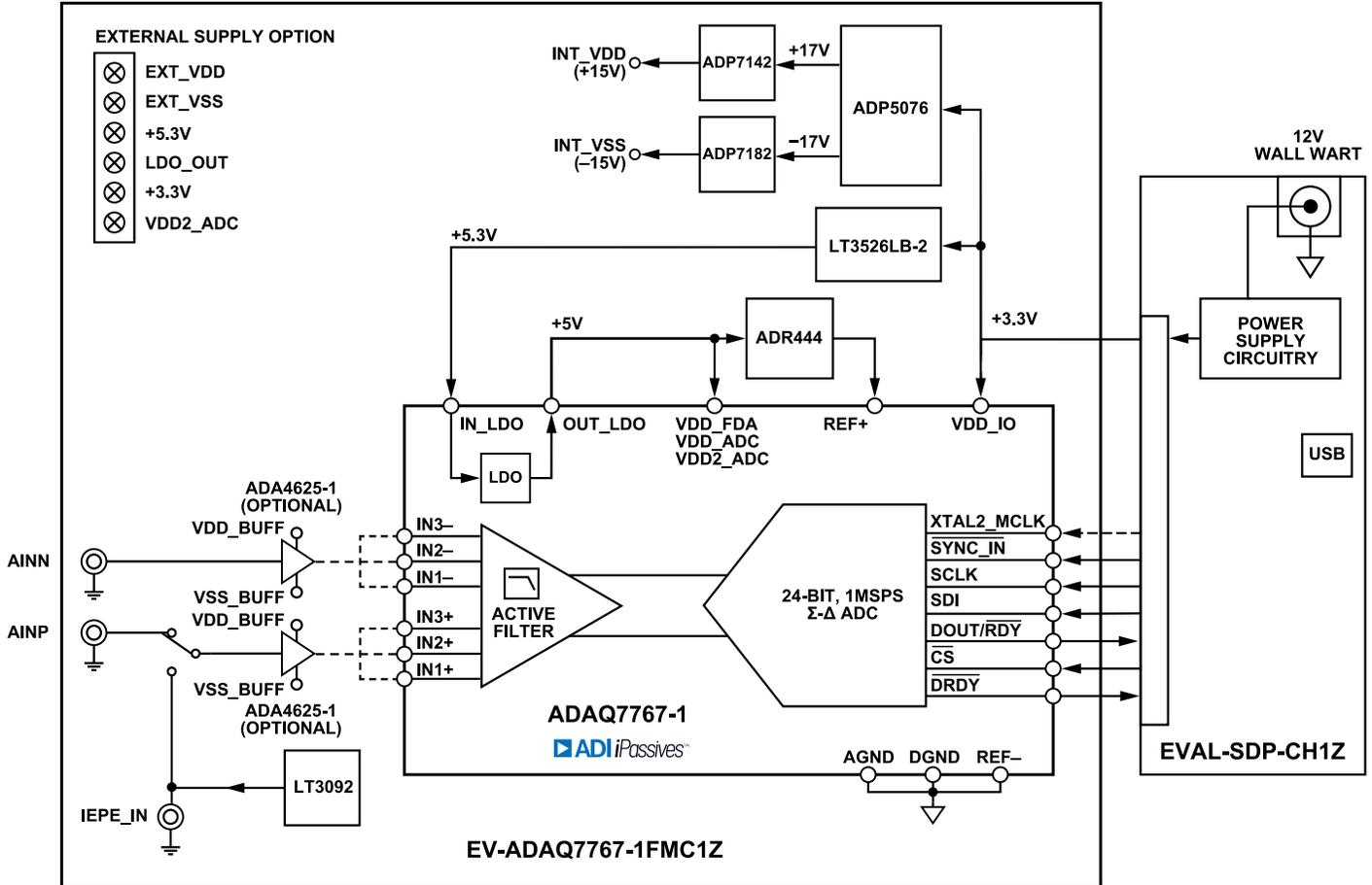
Figure 7. Simplified Evaluation Board Block Diagram
