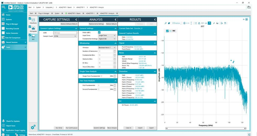
Figure 24. ADAQ7767-1 Board FFT with Shorted Inputs
