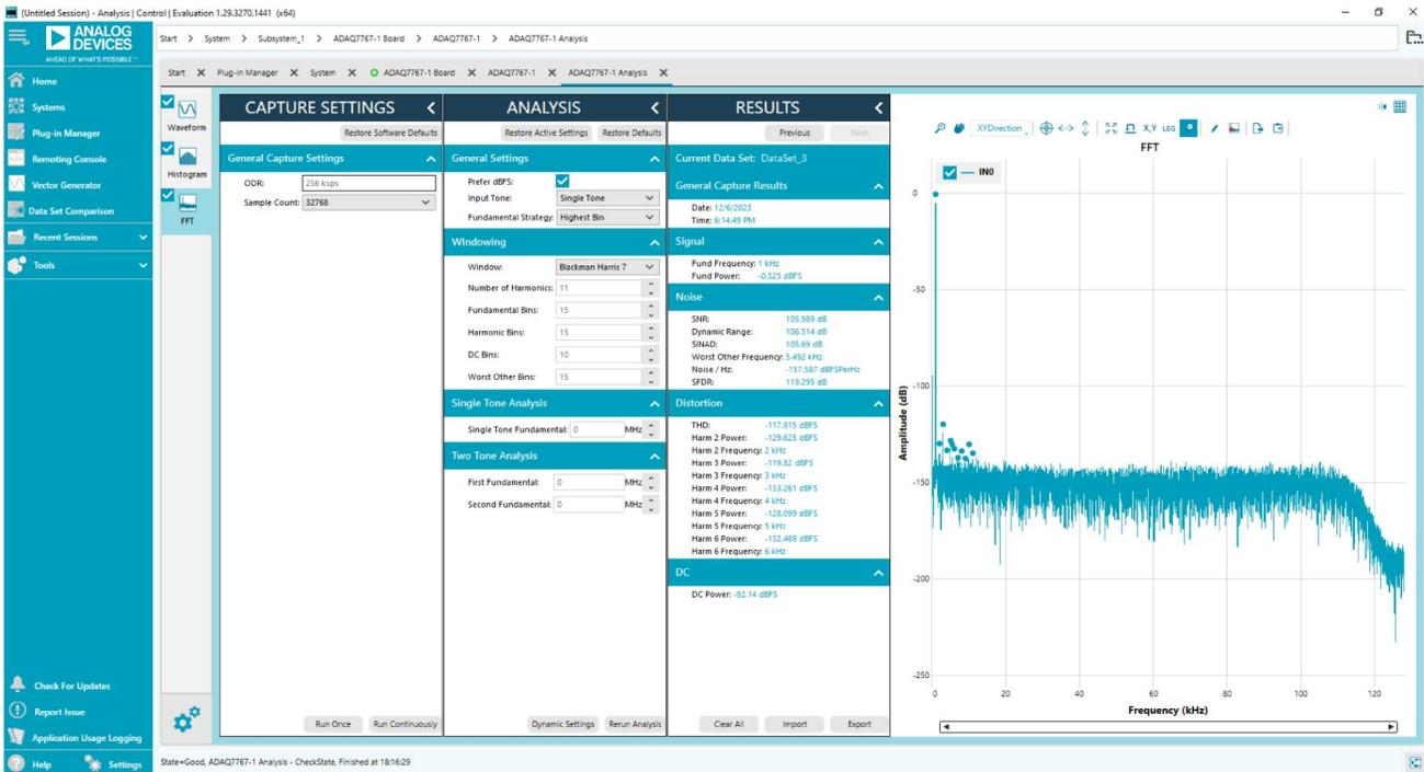
Figure 3. FFT of 10.6 V<sub>p</sub>, a 1 kHz Fully Differential Signal Applied to IN2+ and IN2- Pins of the ADAQ7767-1
