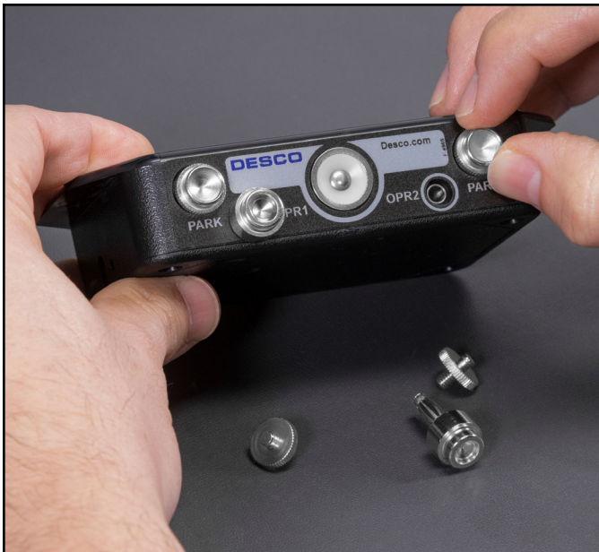
Figure 7. Installing the 10 mm snap adapters to the 19656 Dual Operator Continuous Monitor
