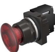
30mm BlackMax, Epoxy Coated Corrosion Resistant Complete Metal Unit Illuminated Push-Pull Operator Full Voltage, 24V AC/DC Incandescent Lamp Mushroom Head Cap Small 1 3/4" (44.5 mm) Plastic, Red 3 Position Momentary UL Listed, CSA Certified NEMA 1,3,3R,4,4X,12,13 & Automotive Standards
