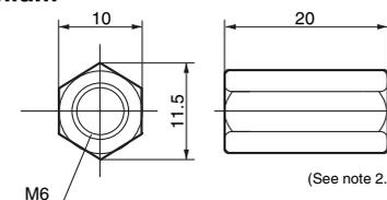
**Note: 1.** Dimension when mounting Electrodes.
