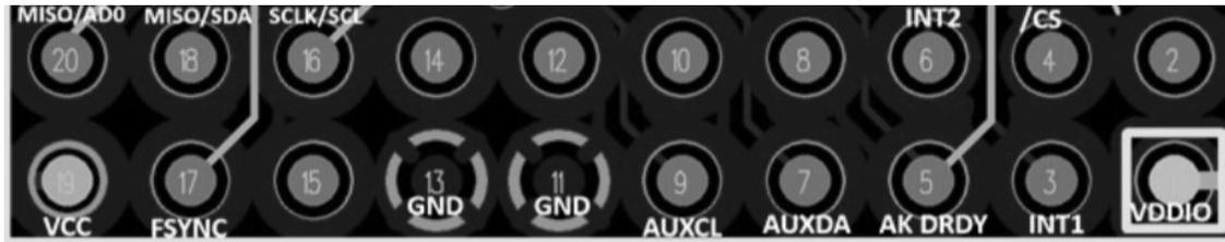
Figure 4. Pin out of CN1 (Connector to EVB)
