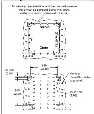
In order for Xinger surface mount delay lines to work optimally, there must be 50Ω transmission lines leading to and from all of the RF ports. Also, there must be a very good ground plane under the part with a number of plated thru holes to ensure proper electrical performance. If any of these conditions are not satisfied, insertion loss, average delay and VSWR may not meet published specifications.
