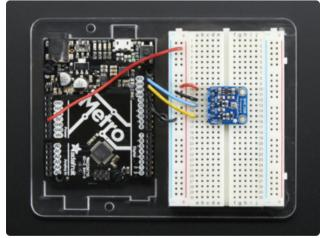
Connect **Vin** to the power supply, 3-5V is fine. Use the same voltage that the microcontroller logic is based off of. For most Arduinos, that is 5V Connect **GND** to common power/data ground
