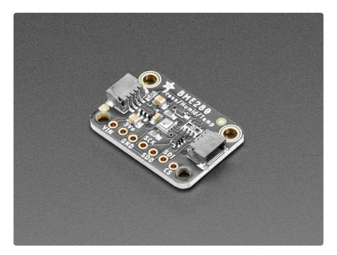
Bosch has stepped up their game with their new BME280 sensor, an environmental sensor with temperature, barometric pressure and humidity! This sensor is great for all sorts of weather/environmental sensing and can even be used in both I2C and SPI!
