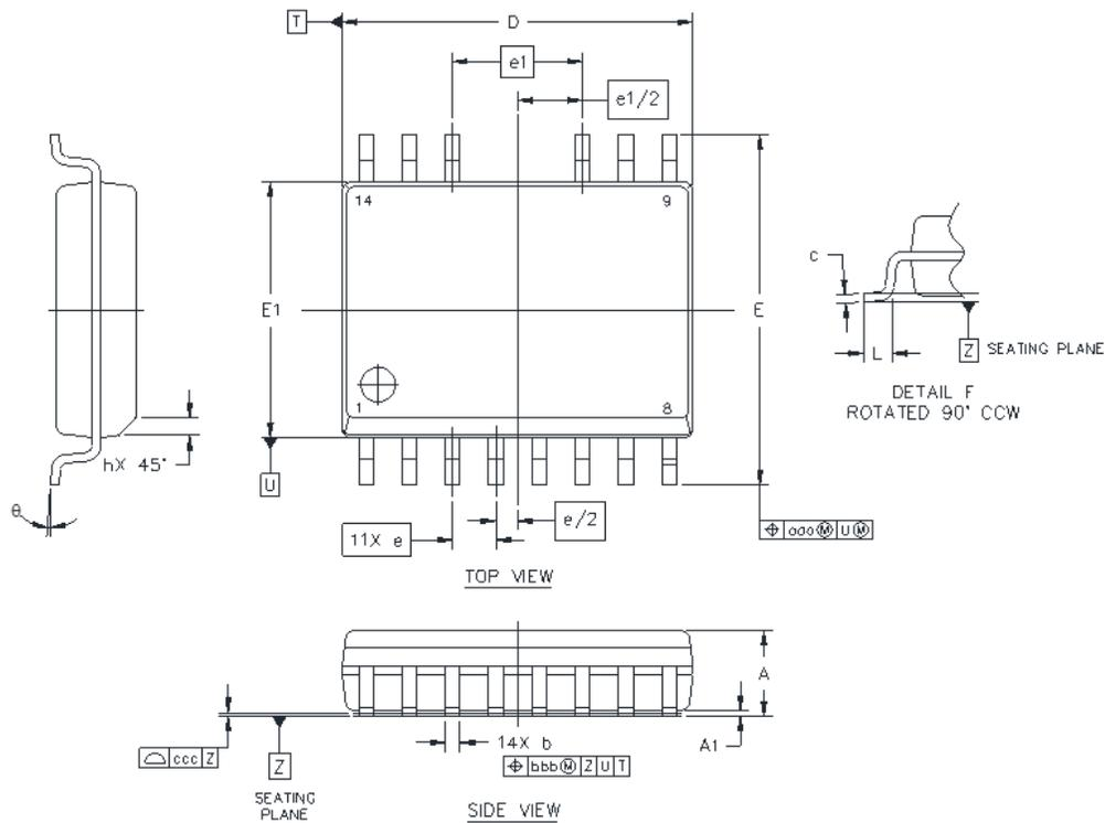
**Figure 7.4. 14-Pin Small Outline Integrated Circuit (SOIC) Package**
