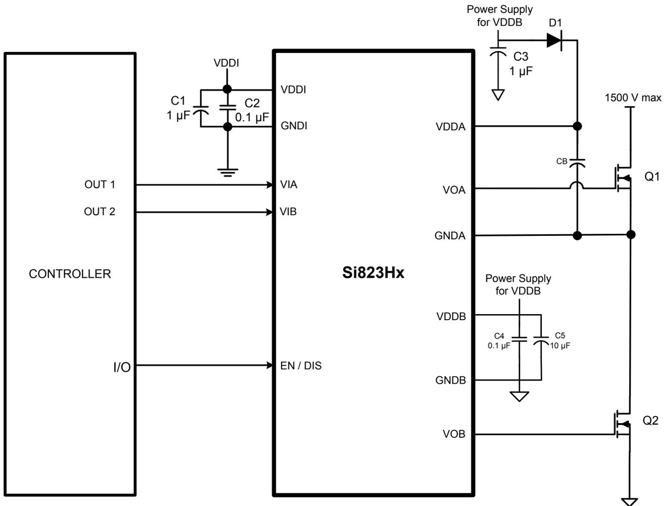
Figure 3.4. Si823H1/2/3/5/6/7 with EN/DIS Pin Application Diagram
