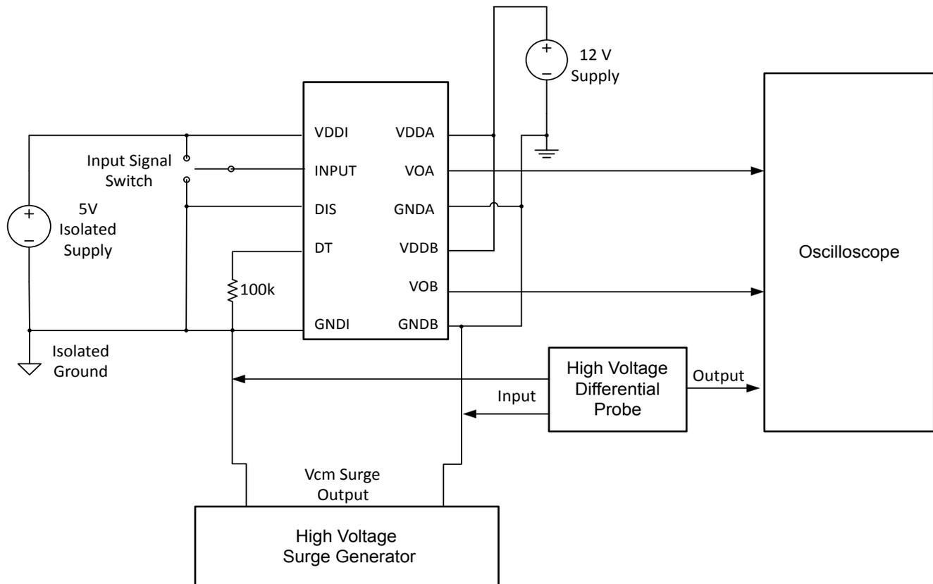
**Figure 4.1. Common Mode Transient Immunity (CMTI) Test Circuit**
