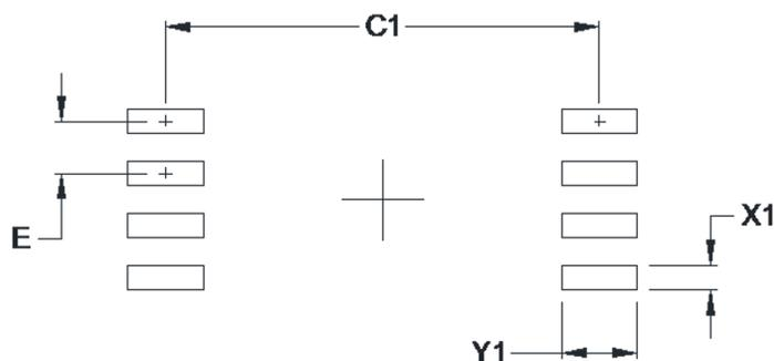
Figure 8.2. 8-Pin Wide Body Stretched SOIC Land Pattern
