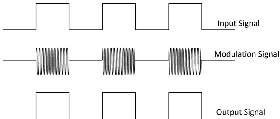
**Figure 2.2. Modulation Scheme**
