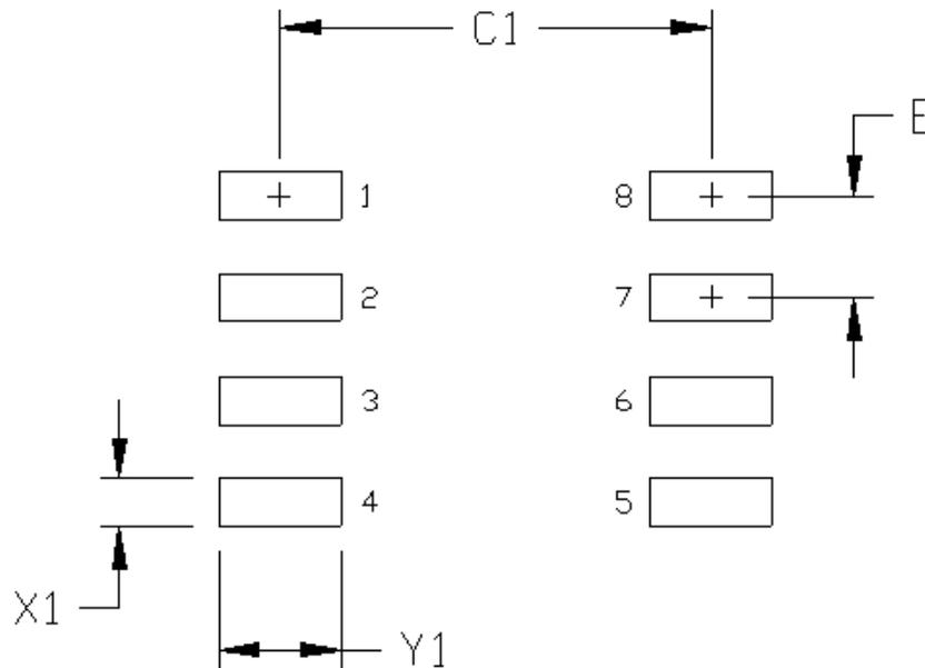
Figure 8.1. 8-Pin Narrow Body SOIC Land Pattern
