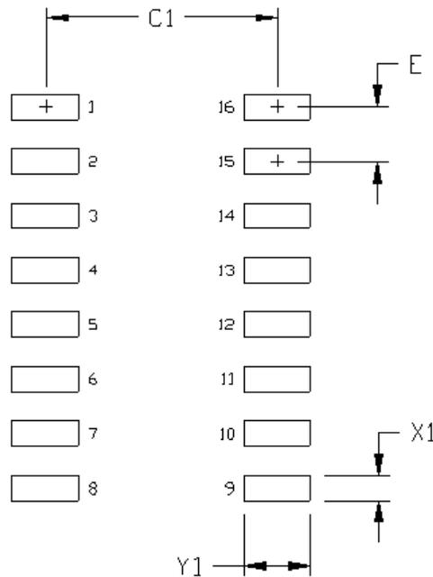
**Figure 8.3. 16-Pin Narrow Body SOIC PCB Land Pattern**
