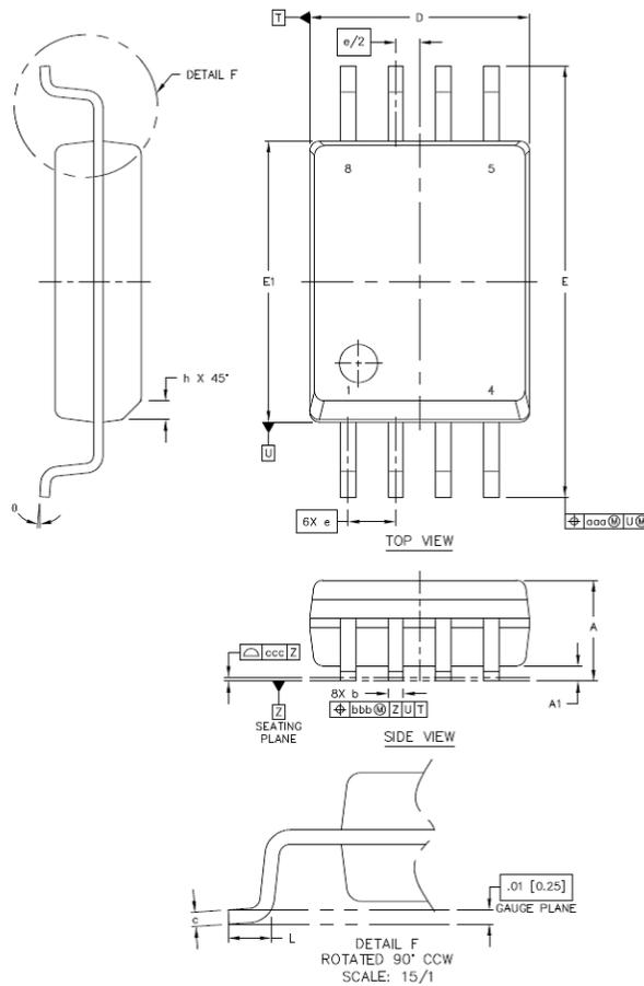
**Figure 7.2. 8-Pin Wide Body Stretched SOIC Package**
