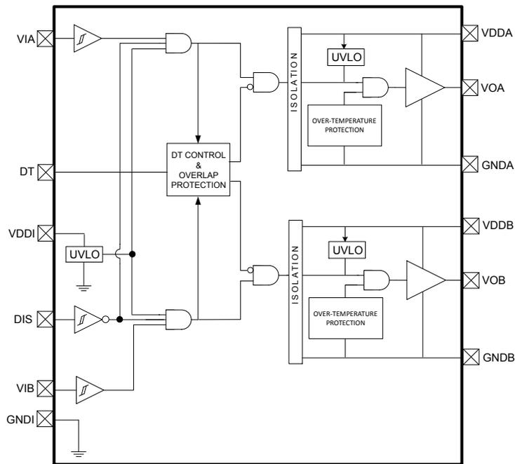
Figure 5.4. Si823H1/3 HS/LS Isolated Drivers with DIS
