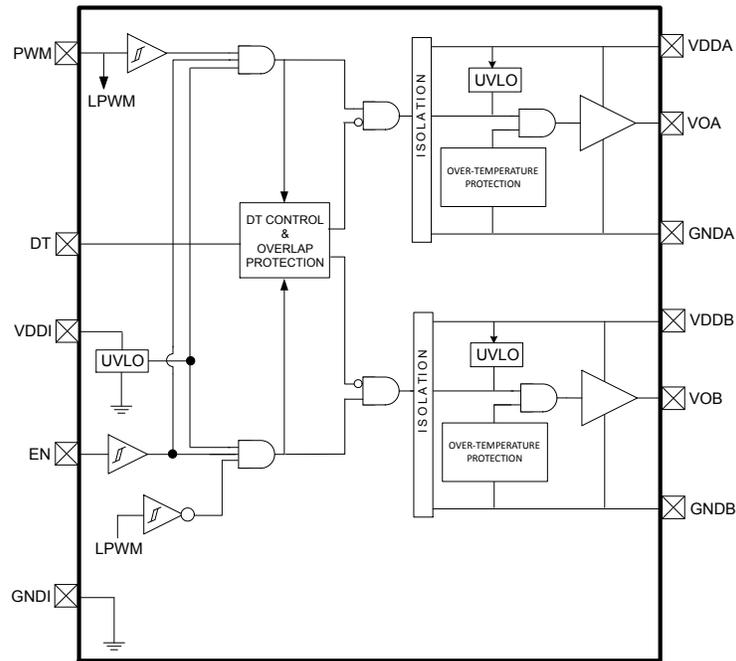
Figure 5.5. Si823H4 Single-Input Isolated Drivers with EN
