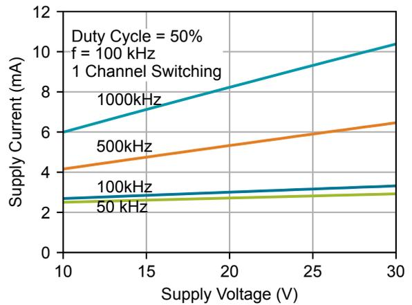
Figure 4.9. Supply Current vs. Supply Voltage ( $C_L = 100$  pF)
