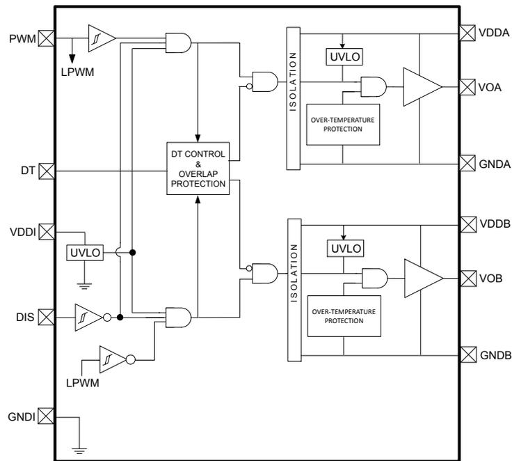
Figure 5.6. Si823H8 Single-Input Isolated Drivers with DIS
