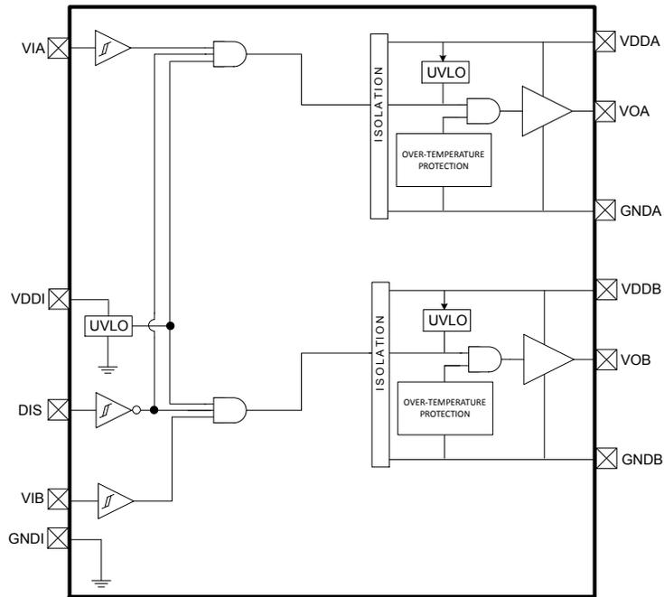
**Figure 5.7. Si823H6 Dual Isolated Drivers with DIS**
