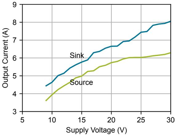
Figure 4.10. Peak Output Current vs. Supply Voltage
