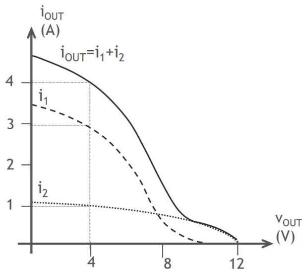
**Figure 2.9. Pull-Up Current Characteristics, VDD = 12 V**
