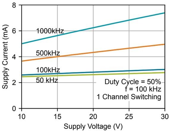
Figure 4.8. Supply Current vs. Supply Voltage ( $C_L = 0$  pF)
