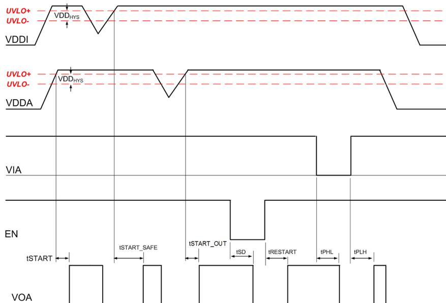
**Figure 2.5. Si823H7 (Delayed Startup Time of t<sub>START\_SAFE</sub>) Device Behavior During Normal Operation and Shutdown**
