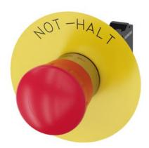
EMERGENCY STOP mushroom-type actuator, 22 mm, round, metal, shiny, red, 40 mm, positive latching, according to EN ISO 13850, rotate-to-unlatch, with yellow backing plate, inscription: NOT-HALT, with holder, 1 NC, spring-type terminal, Z=20-unit packaging
