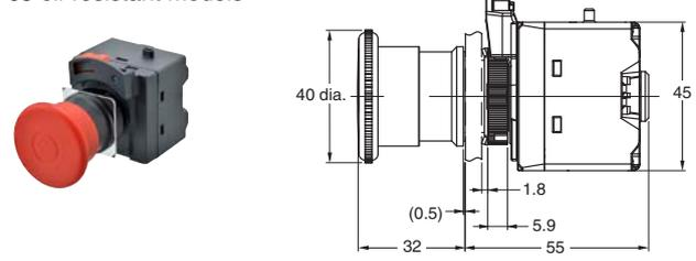
**Note:** The dimensions the same even if the Operation Unit is replaced with the A22NE-MR□-N or the A22NE-MR□-N-RD.
