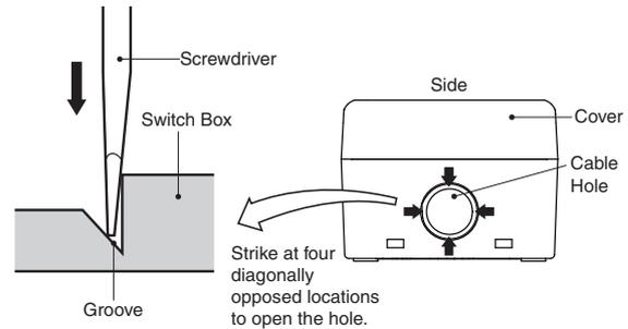
**(3) Securing the Connector Cable**
