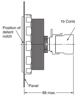
**Screw Terminal Block Type Mounting a 2-pole Switch Unit \***
