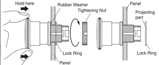
1. When the panel cutout dimension is 25 dia., remove the supplied rubber washer and mount the 25-dia. Ring as shown below. (Since the A22Z-R25 is not attached to the main body, order separately.) When using a Legend Plate (Order Separately), do not remove the rubber washer.
