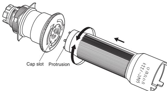
**Installing/Replacing the LED Lamp**
