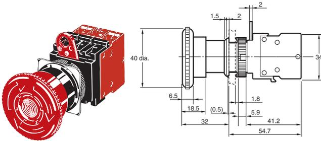
Switch dimensions when mounted to a 2NO (2NC) one-piece switch block
