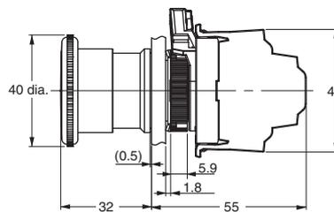
**Note:** Unless otherwise specified, a tolerance of  $\pm 0.8$  mm applies to all dimensions.
