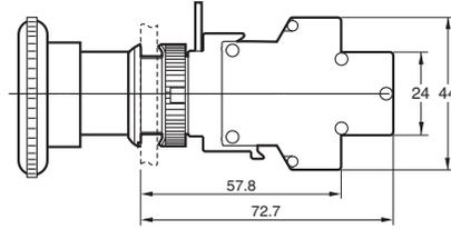
**Note:** The operation unit is an example for the A22E-M.
