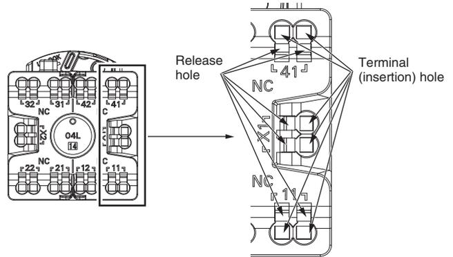
**Connecting Wires with Ferrules and Solid Wires**
