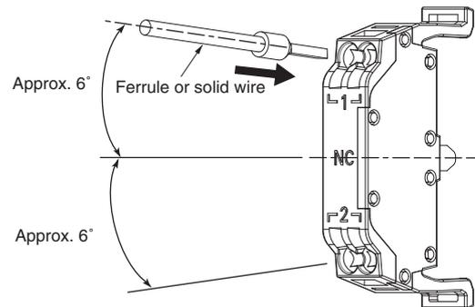
The wiring for the Lighting Unit and Switch Block (2 contacts) are the same as for the Switch Block (1 contact) shown in the above illustration.
