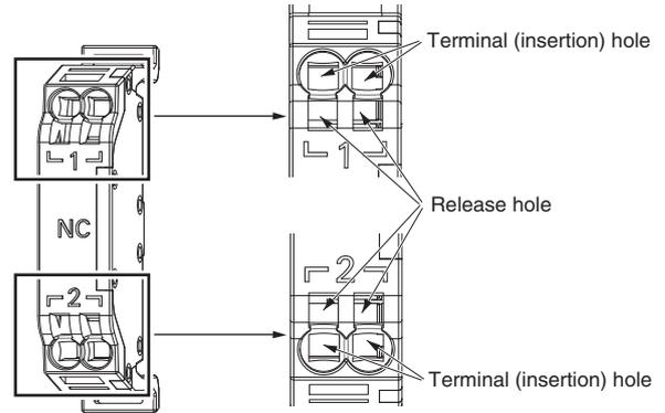
**Connecting Wires with Ferrules and Solid Wires**
