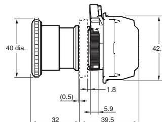
**Note:** The dimensions are the same even if the Operation Unit is replaced with the A22NE-MR□-N or the A22NE-MR□-N-RD.
