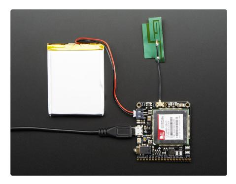
Then press the small **KEY** button next to the battery & cell antenna for 5 seconds. Then the computer will recognize a multi-type USB connection. <a href="Install the drivers">Install the drivers (https://adafru.it/jFn)</a>
