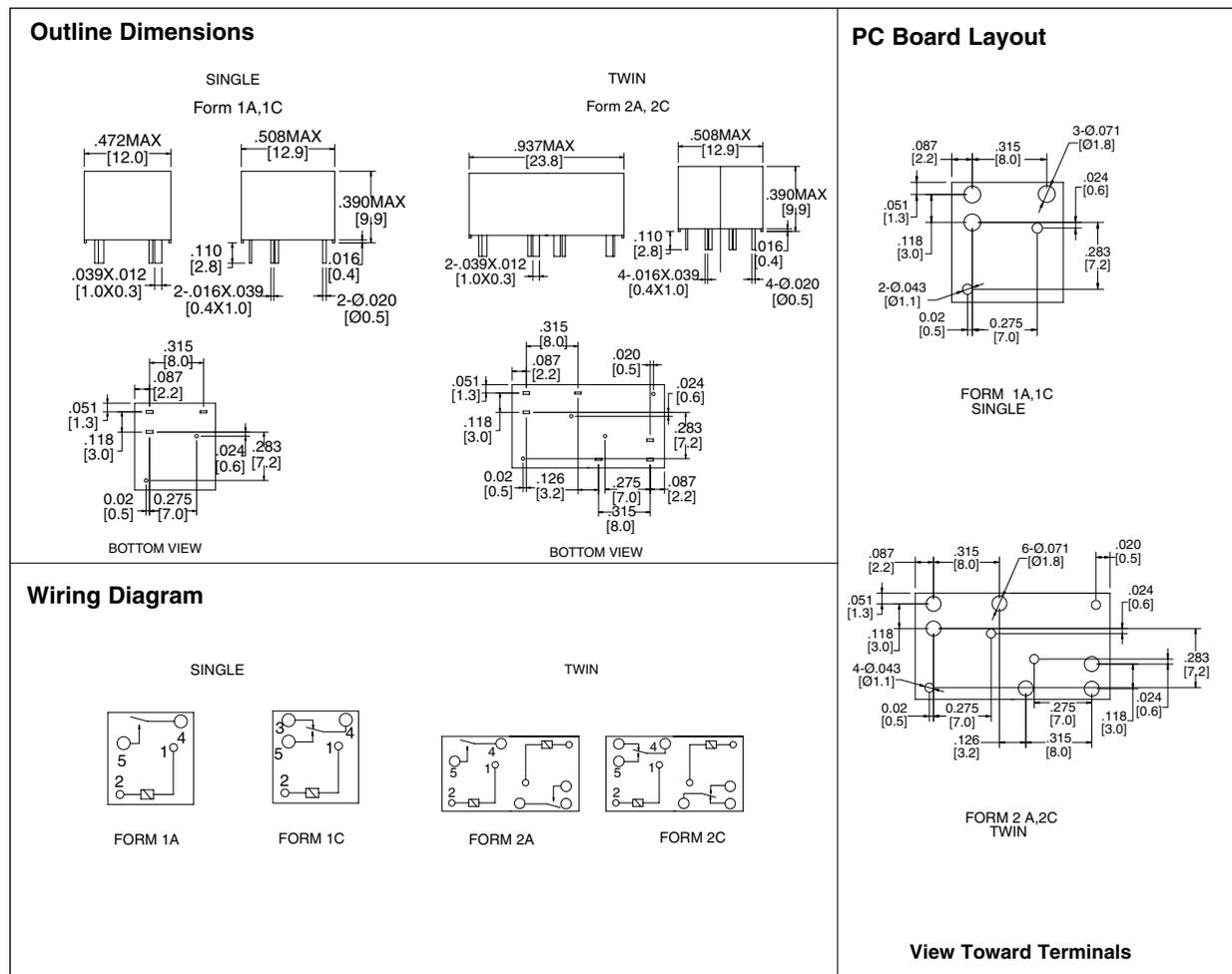
Dimensions in inches with millimeters in brackets below. Tolerance:  $\pm .010$ "
