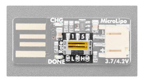
On the MicroLipo v2, there is a switch in the center of the board that replaces the jumper for changing between 100mA and 500mA charging modes. 100mA is labeled with 1 above the switch and  $\bf L$  below the switch (for low mode). 500mA is labeled with 5 above the switch and  $\bf H$  below the switch (for high mode).
