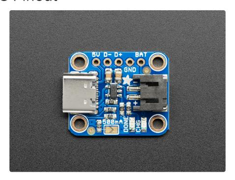
The USB-C Micro-Lipo charger is special. We've exposed the data lines so you can use it both as a USB-C breakout and a Micro-Lipo charger. Since there's a little more to it, we've included the pinouts here. Let's take a look!
