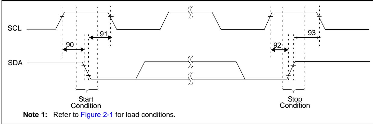
**FIGURE 2-6: I<sup>2</sup>C™ BUS DATA TIMING**
