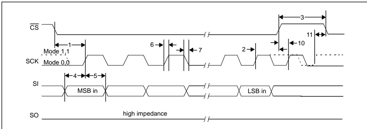
**FIGURE 2-8: SPI OUTPUT TIMING**
