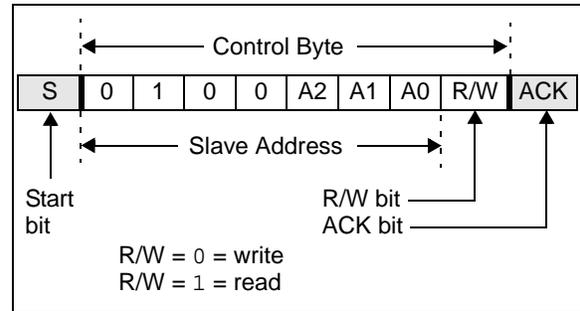
**FIGURE 1-7: SPI CONTROL BYTE FORMAT**
