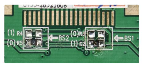
(If you solder and re-solder the resistors 10 times like I did while figuring out all the setting and wiring, you'll get a kinda messy/fluxy look like the above! In that case you can clean up with some IPA wipes. Or just revel in your punk soldering job)
