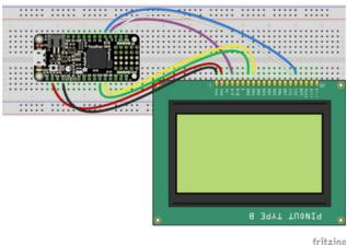
OLED Pin #1 to Microcontroller GND OLED Pin #2 to Microcontroller 3.3V OLED Pin #4 to Microcontroller D6 OLED Pin #7 to Microcontroller SCK OLED Pin #8 to Microcontroller MOSI OLED Pin #15 to Microcontroller D5 OLED Pin #16 to Microcontroller D9
