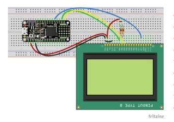
OLED Pin #1 to Microcontroller GND OLED Pin #2 to Microcontroller 3.3V OLED Pin #4 to Microcontroller GND OLED Pin #7 to Microcontroller SCL 10K resistor from SCL to 3.3V OLED Pin #8 to Microcontroller SDA OLED Pin #9 to Microcontroller SDA 10K resistor from SDA to 3.3V OLED Pin #16 to Microcontroller D9
