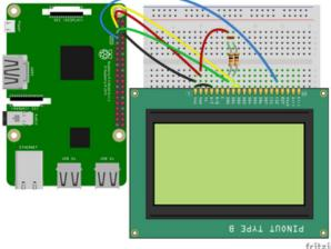
OLED Pin #1 to Raspberry Pi GND OLED Pin #2 to Raspberry Pi 3.3V OLED Pin #4 to Raspberry Pi GND OLED Pin #7 to Raspberry Pi SCL 10K resistor from SCL to 3.3V OLED Pin #8 to Raspberry Pi SDA OLED Pin #9 to Raspberry Pi SDA 10K resistor from SDA to 3.3V OLED Pin #16 to Raspberry Pi GPIO 4
