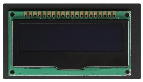
The pins on these modules are not well marked, but the one on left is #1 and the pins increment in order until the one on the very right, #20
