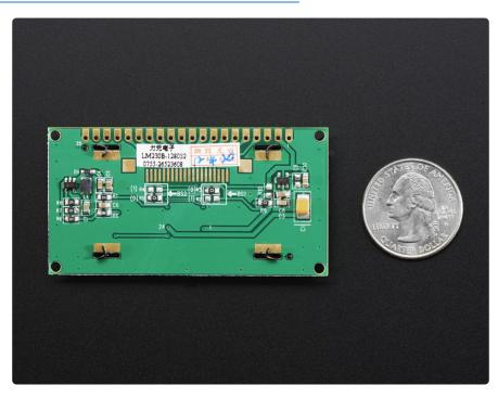
Getting started is easy! We have a detailed tutorial and example code in the form of an Arduino library for text and graphics. (https://adafru.it/j6a) You'll need a microcontroller with more than 512 bytes of RAM since the display must be buffered. The library can print text, bitmaps, pixels, rectangles, circles and lines. It uses 512 bytes of RAM since it needs to buffer the entire display but its very fast! The code is simple to adapt to any other microcontroller.
