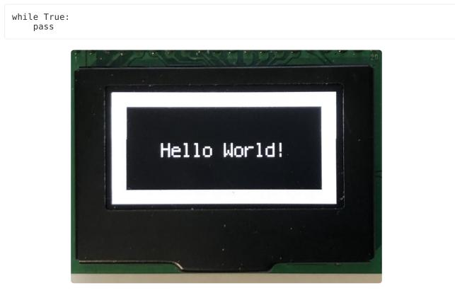
If you have the 2.3" 128x32 OLED Display, here's what the final output looks like with the height set to 32 and the border size set to 5:
