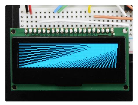
The power requirements depend a little on how much of the display is lit but on average the display uses about 50mA from the 3.3V supply. Built into the OLED driver is a simple switch-cap charge pump that turns 3.3V into a high voltage drive for the OLEDs.
