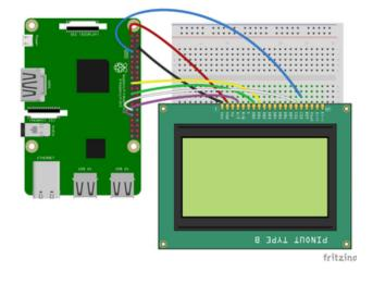
OLED Pin #1 to Raspberry Pi GND OLED Pin #2 to Raspberry Pi 3.3V OLED Pin #4 to Raspberry Pi GPIO 6 OLED Pin #7 to Raspberry Pi SCK OLED Pin #8 to Raspberry Pi MOSI OLED Pin #15 to Raspberry Pi GPIO 5 OLED Pin #16 to Raspberry Pi GPIO 4
