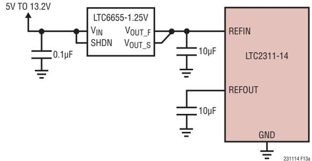
Figure 13a. LTC2311-14 with an External REFIN Voltage
