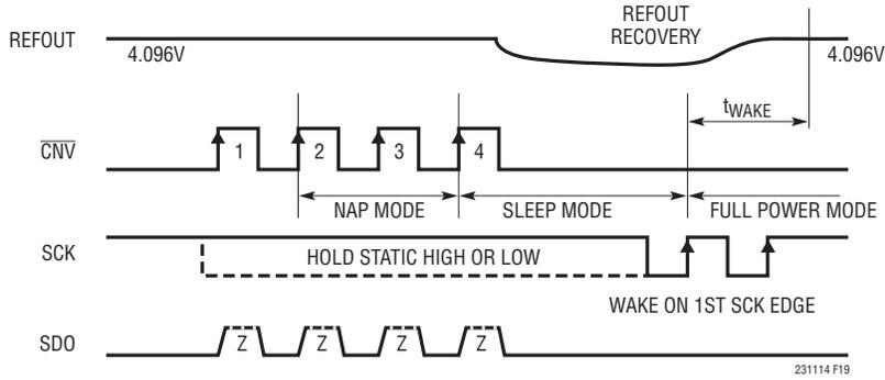
Figure 19. CMOS Mode SLEEP and WAKE Using SCK
