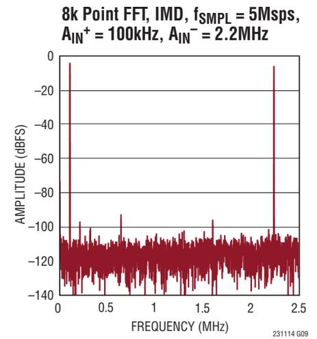
**TYPICAL PERFORMANCE CHARACTERISTICS**  $T_A = 25^\circ\text{C}$ ,  $V_{DD} = 5\text{V}$ ,  $OV_{DD} = 2.5\text{V}$ ,  $REF_{OUT} = 4.096\text{V}$ ,  $f_{SAMPL} = 5\text{Msps}$ , unless otherwise noted.
