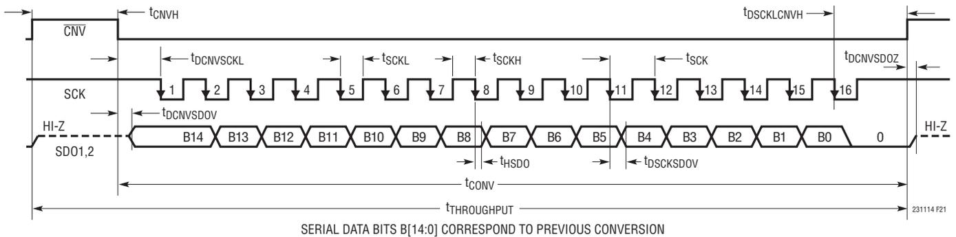
Figure 21. LTC2311-14 Timing Diagram, CMOS, LVDS I/O Modes
