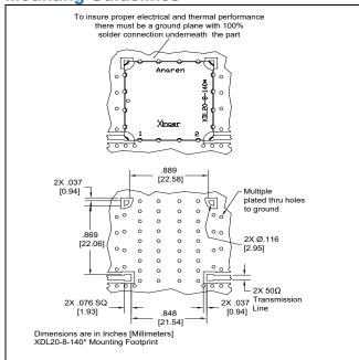
In order for Xinger surface mount delay lines to work optimally, there must be  $50\Omega$  transmission lines leading to and from all of the RF ports. Also, there must be a very good ground plane under the part with a number of plated thru holes to ensure proper electrical performance. If any of these conditions are not satisfied, insertion loss, average delay and VSWR may not meet published specifications.
