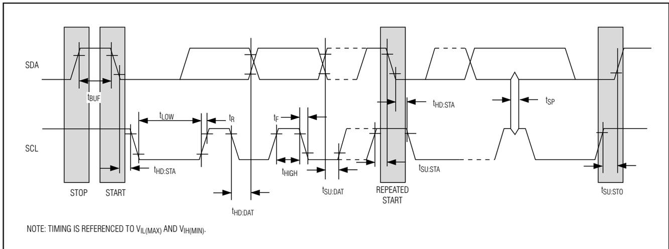
Figure 4. I<sup>2</sup>C Timing Diagram
