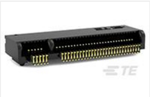
TE Part #1-2199119-6 M.2 0.5PITCH 3.2H KEY M 30U" AU
