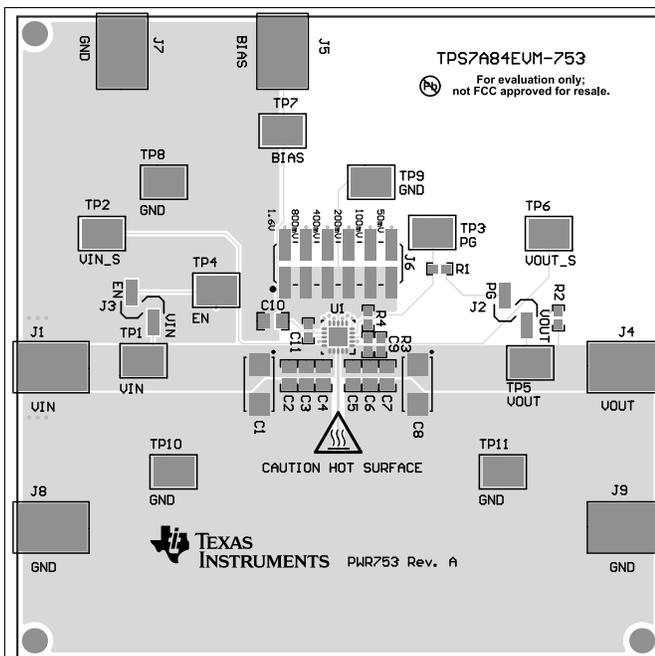
Figure 1. Assembly Layer
