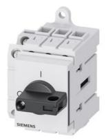
Load disconnector 3LD3, Iu 16 A Main switch 3-pole Rated operating capacity at AC-23 A at 400V 7.5kW Installation in distribution boards, Basic switch with selector knob black with auxiliary switch 10E + 1S
