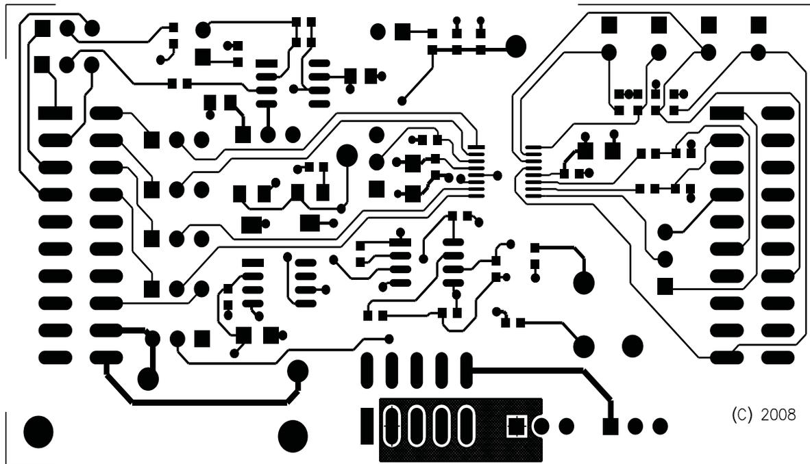
Figure 3. Layer 1 (Top Signal Plane)
