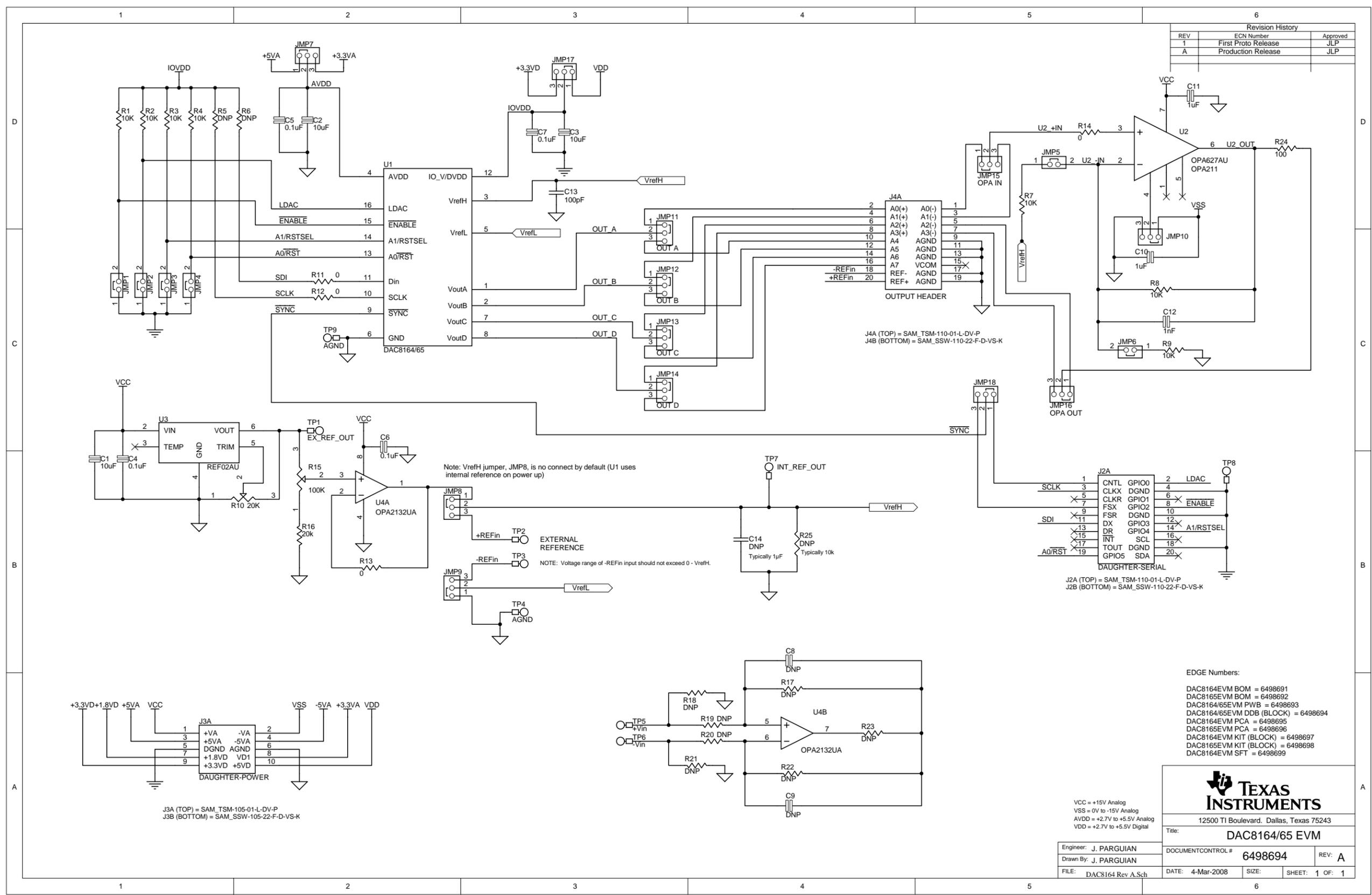
Note: VrefH jumper, JMP8, is no connect by default (U1 uses internal reference on power up)
