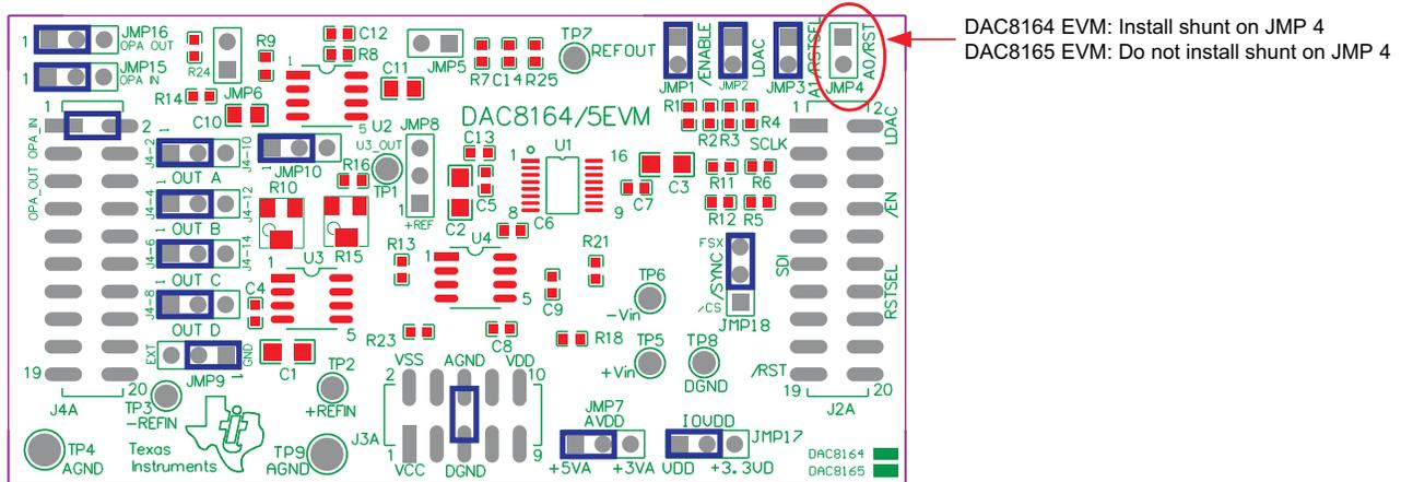
**Figure 9. DAC8164/65EVM Default Jumper Configuration**
