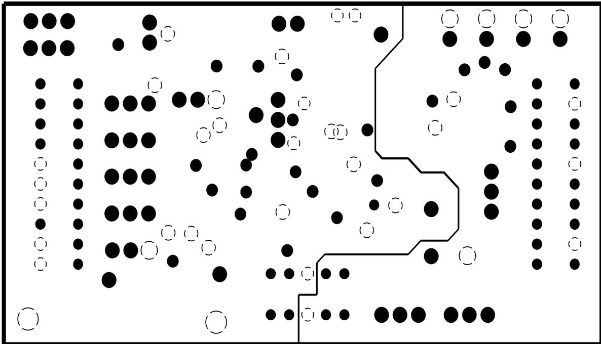
Figure 4. Layer 2 (Ground Plane)
