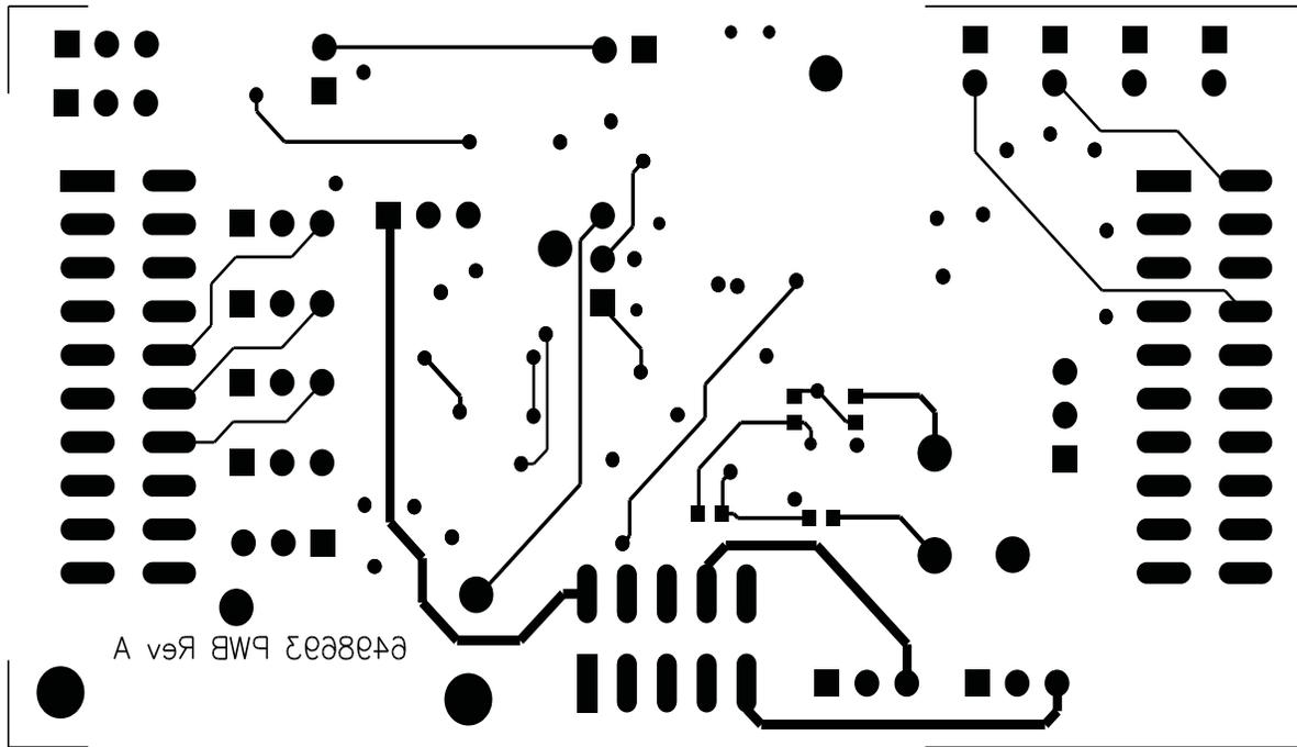
Figure 6. Layer 4 (Bottom Signal Plane)
