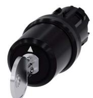
Key-operated switch BKS, 22 mm, round, plastic, Lock No. E9 (VW), without key, 3 switch positions I-O-II, latching, actuating angle  $2x45^{\circ}$ , 10:30h/12h/13:30h, Key removal I+O+II Z=50-unit packaging
