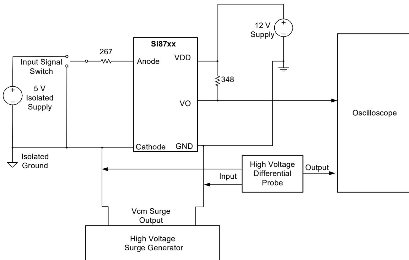
**Figure 2. Common Mode Transient Immunity Characterization Circuit**
