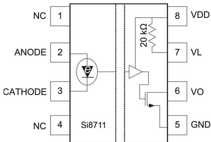
Figure 15. Pin Configuration
