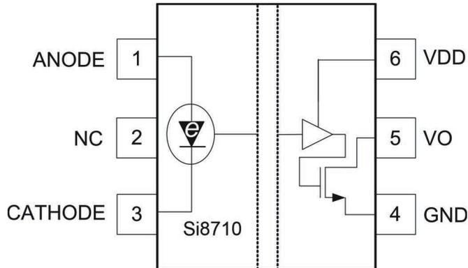
Figure 14. Pin Configuration
