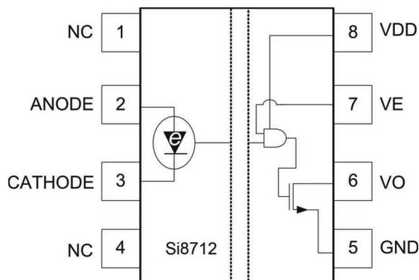
Figure 13. Pin Configuration
