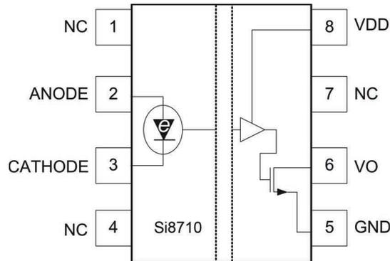
**Figure 12. Pin Configuration**
