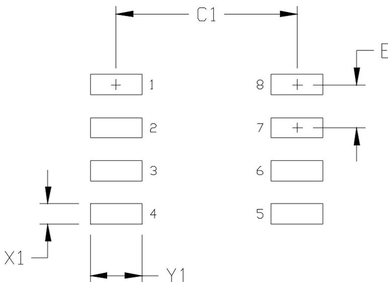
**Figure 17. 8-Pin Narrow Body SOIC Land Pattern**
