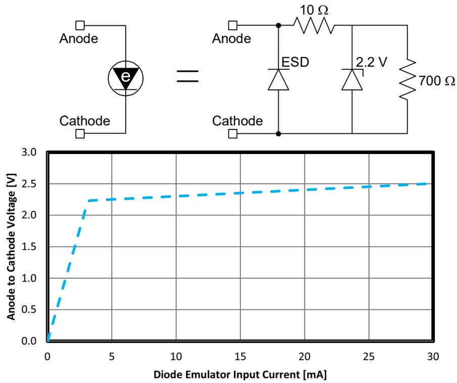
**Figure 1. Diode Emulator Model and I-V Curve**
