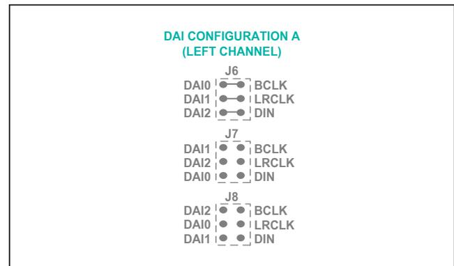
Figure 3. DAI Configuration A (Left Channel for I<sup>2</sup>S/Left-Justified Operation)
