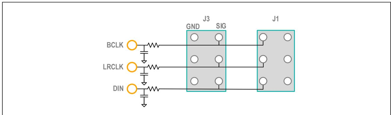
Figure 4. MAX98360 DAI Interface Headers (PCM)
