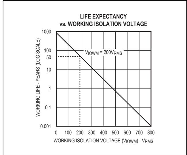
Figure 4. Life Expectancy vs. Working Isolation Voltage
