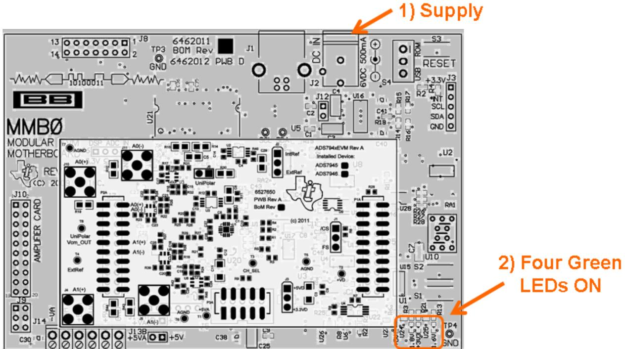
Figure 8. Powering Up ADS794xEVM-PDK
