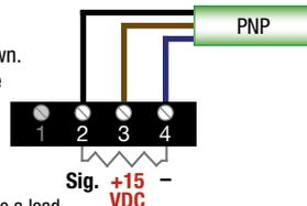
Some sensors may require a load resistor. See sensor mfr. specs. and Sensor Load section at left.
