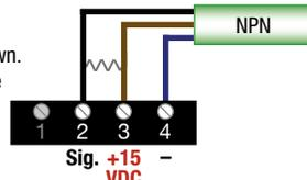
Some sensors may require a load resistor. See sensor mfr. specs. and Sensor Load section at left.
