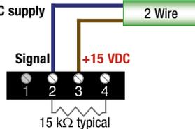
Some sensors may require a bleed resistor. See sensor mfr. specs.
