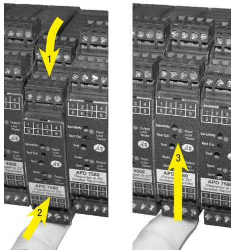
1. Tilt front of module downward and position against DIN rail.
