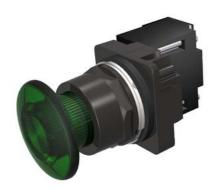
30mm BlackMax, Epoxy Coated Corrosion Resistant Complete Metal Unit Illuminated Push-Pull Operator Full Voltage, 6V AC/DC Incandescent Lamp Mushroom Head Cap Small 1 3/4" (44.5 mm) Plastic, Green 3 Position Pull-Momentary/Push-Maintained UL Listed, CSA Certified NEMA 1,3,3R,4,4X,12,13 & Automotive Standards
