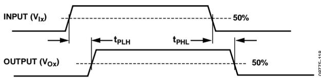
Figure 24. Propagation Delay Parameters
