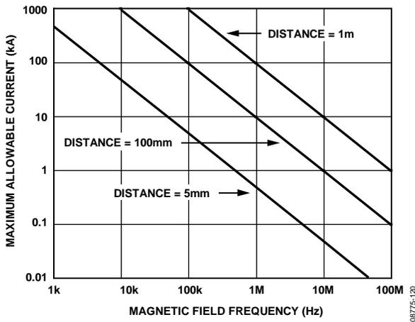
Figure 26. Maximum Allowable Current for Various Current-to-ADuM620x Spacings
