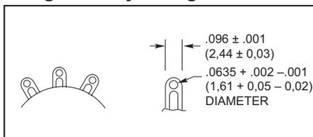
The gold-plated terminal features a slot to accept wires in addition to the conventional wire hole.
