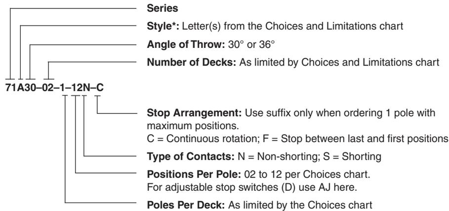
\* All rotary switches that are required to have military designated markings and testing adhering to MIL-DTL-3786 are to be ordered by specifying the military part number identified on the appropriate slash sheet.
