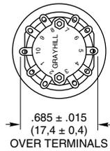
Note: Switch/key positions are not aligned with terminal positions.
