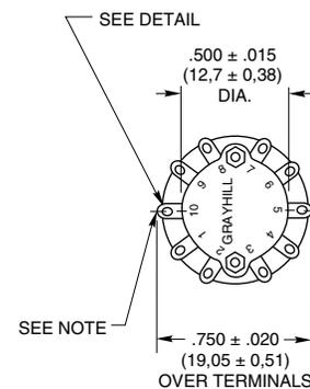
**Note:** Common location for a single pole per deck switch. For common location on multiple switches see circuit diagrams.
