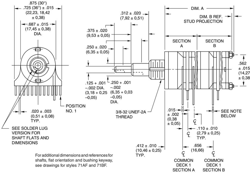
For additional dimensions and references for shafts, flat orientation and bushing keyway, see drawings for styles 71AF and 71BF.
