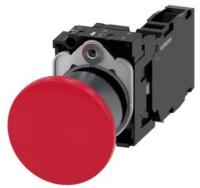
Mushroom pushbutton, 22 mm, round, plastic with metal front ring, red, 40mm, latching, pull-to-unlatch mechanism, with holder, 1 NO+1 NC, screw terminal, with laser labeling, lower case
