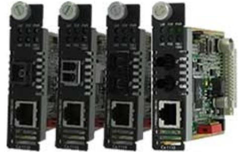
Installed in a high density Perle Media Converter Chassis, Perle's feature rich **Managed Fast Ethernet Media Converter Modules** transparently connect UTP copper to fiber. Our fast ethernet media converters provide an economical path to extend the distance of an existing network, the life of non-fiber based equipment, or the distance between two devices.
