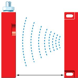
Encapsulated in the MA Series is a unique high-power industrial reed which is de-rated by a non-resetable overload protection circuit depending on switch type. On presenting the actuator to the switch, the high intensity magnetic field from the actuator causes the contacts to close. On removing the actuator (opening the door), the safety contacts open, isolating the machine.
