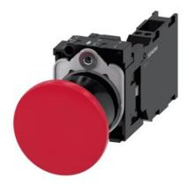
Mushroom pushbutton, 22 mm, round, plastic, red, 40mm, latching, pull-to-unlatch mechanism, with holder, 1 NO+1 NC, spring-type terminal, with laser labeling, inscription or symbol Customer-specific selection with SIRIUS ACT configurator (CIN)
