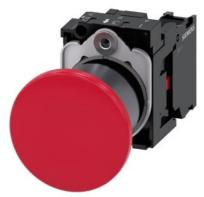
Mushroom pushbutton, 22 mm, round, plastic with metal front ring, red, 40mm, latching, pull-to-unlatch mechanism, with holder, 1 NC, screw terminal, with laser labeling, upper case and lower case, always upper case at the beginning of the word
