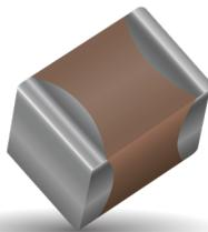
The X7R dielectric is the most popular of the intermediate EIA class II materials due to its relative temperature stability. While the capacitance change is non-linear, temperature variation is within  $\pm 15\%$  from  $-55^\circ\text{C}$  to  $+125^\circ\text{C}$ .
