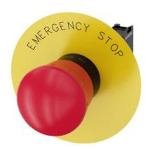
EMERGENCY STOP mushroom pushbutton, 22 mm, round, plastic, red, 40 mm, positive latching, acc. to EN ISO 13850, rotate-to-unlatch, with yellow backing plate, inscription: EMERGENCY STOP, with holder, 1 NC, screw terminal, Z=20-unit packaging
