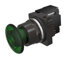
30mm BlackMax, Epoxy Coated Corrosion Resistant Complete Metal Unit Illuminated Push-Pull Operator Full Voltage, 12V AC/DC Incandescent Lamp Mushroom Head Cap Small 1 3/4" (44.5 mm) Plastic, Green 3 Position Momentary UL Listed, CSA Certified NEMA 1,3,3R,4,4X,12,13 & Automotive Standards
