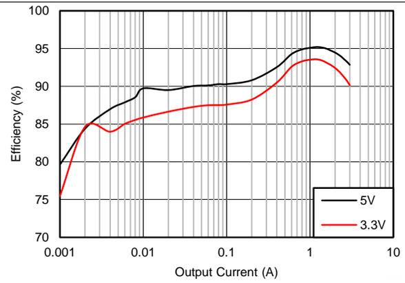
**Figure 6. Efficiency:  $V_{IN} = 12\text{ V}$ ,  $f_{sw} = 400\text{ kHz}$**
