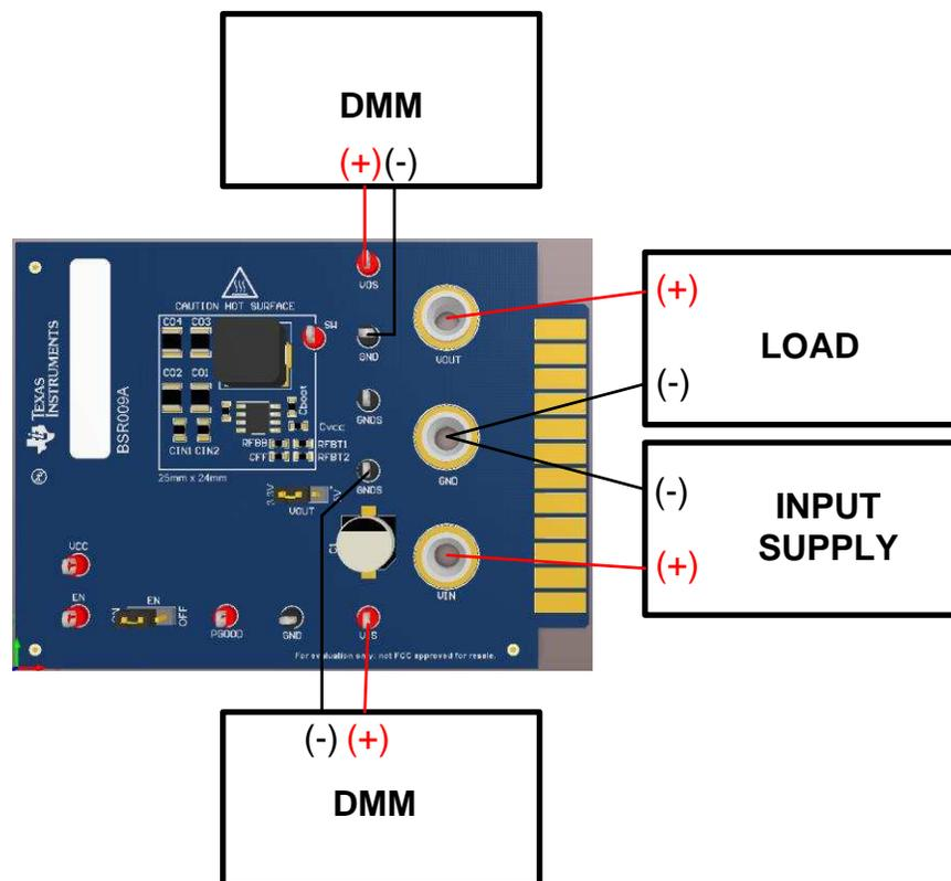
Figure 1. EVM Board Connections
