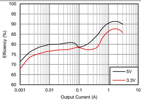
**Figure 5. Efficiency:  $V_{IN} = 12\text{ V}$ ,  $f_{sw} = 2.1\text{ MHz}$**
