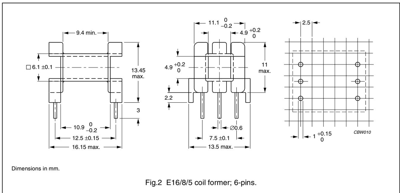
**Winding data and area product for 6-pins E16/8/5 coil former**
