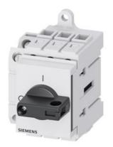
Load disconnector 3LD3, lu 25 A Main switch 3-pole Rated operating capacity at AC-23 A at 400V 9.0kW Installation in distribution boards, Basic switch with selector knob black with auxiliary switch 10E + 1S
