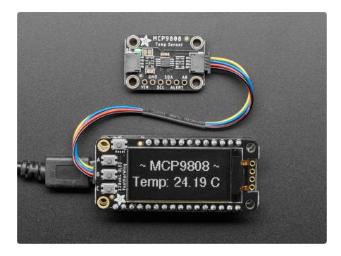
This I2C digital temperature sensor is one of the more accurate/precise we've ever seen, with a typical accuracy of  $\pm 0.25^{\circ}$ C over the sensor's -40°C to +125°C range and precision of +0.0625°C. They work great with any microcontroller using standard i2c. There are 3 address pins so you can connect up to 8 to a single I2C bus without address collisions. Best of all, a wide voltage range makes is usable with 2.7V to 5.5V logic!
