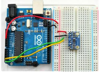
Connect VIN (Vdd) (red wire on the STEMMA QT version) to the power supply, 3V or 5V is fine. Use the same voltage that the microcontroller logic is based off of. For most Arduinos, that is 5V Connect GND (black wire on the STEMMA QT version) to common power/data ground
