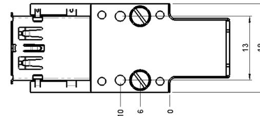
MA033469 USB3 Type-A Test Connector is a 9-pin Test Plug with straight signaling. It is also compatible with USB 2.0 type-A.
