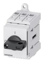
Load disconnector 3LD3, lu 63 A Main switch 3-pole Rated operating capacity at AC-23 A at 400V 22.0 kW Installation in distribution boards, Basic switch with selector knob black
