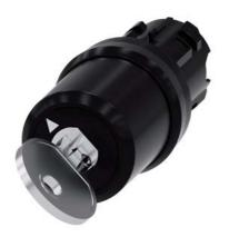
key-operated switch Siemens, 22 mm, round, plastic, lock no. LSG1, with 2 keys, 2 switch positions O-I, latching, actuating angle  $90^\circ$ , 10:30h/13:30h, key removal O, with laser labeling, lower case
