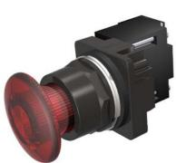
30mm BlackMax, Epoxy Coated Corrosion Resistant Complete Metal Unit Illuminated Push-Pull Operator Full Voltage, 120V AC/DC Incandescent Lamp Mushroom Head Cap Small 1 3/4" (44.5 mm) Plastic, Red 3 Position Momentary UL Listed, CSA Certified NEMA 1,3,3R,4,4X,12,13 & Automotive Standards
