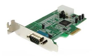
The PEX1S53LP PCI Express Serial Card turns a PCI Express slot into an RS232 (DB9) serial connection.
